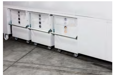
Clamp the chippings container into place
