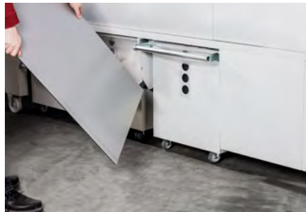
Release the chippings container
