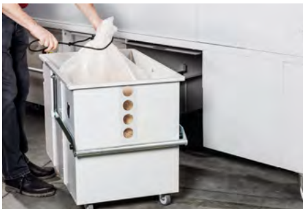
Replace the chippings container
