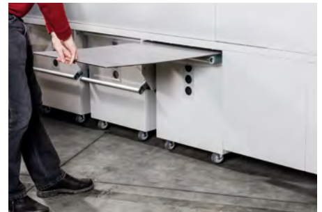
Push in the dust compartment
