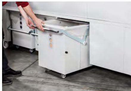
Reinsert the chippings container and remove the dust compartment
